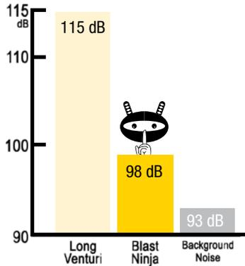
Blast Ninja™ reduces nozzle air exit velocity while maintaining particle velocity – therefore reducing noise production at the source while maintaining blasting production. Oceanit performed many years of extensive fluid dynamic modeling, lab analysis, field trials, and rigorous operator testing in various conditions to arrive at the final Blast Ninja™ product.
