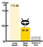
reduces air blast exit velocity while maintaining particle velocity, thus reducing noise while maintaining the abrasive productivity of the nozzle.
