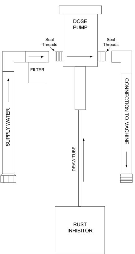
Assemble tubing per diagram below.
